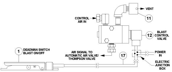
Figure 5.4 – Electric Blast Control System
