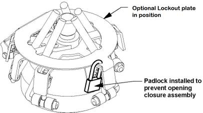
Figure 6.4.2 – Closure Assembly with Halok & Optional Lockout
