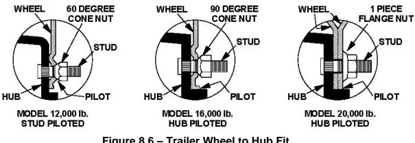
Figure 8.6 – Trailer Wheel to Hub Fit
