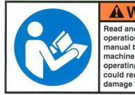
Read and understand the operation and maintenance manual before using this machine. Failure to follow operating instructions could result in injury or damage to equipment.
