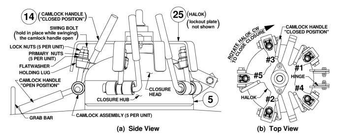
Figure 6.4.1 – Bulk Abrasive Blaster Closure Assembly
