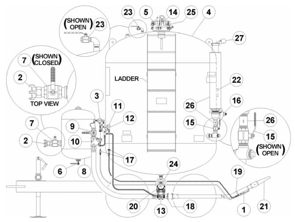
Figure 8.4(a) – Typical Bulk Abrasive Blaster w/CEN
