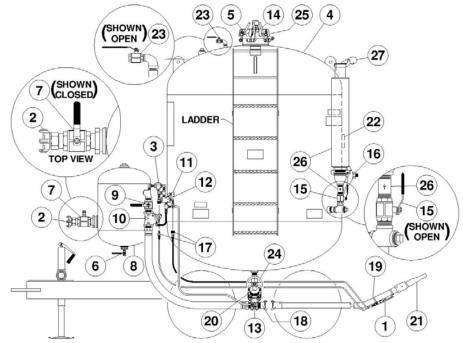
Figure 7.3 – Typical Bulk Abrasive Blaster
