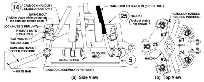
Figure 6.3.1 – Bulk Abrasive Blaster Closure Assembly
