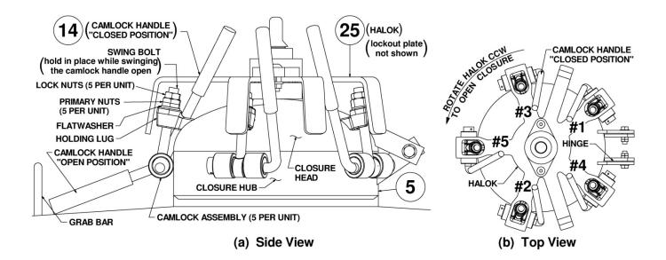
Figure 6.3.2 – Bulk Abrasive Blaster Closure Assembly
