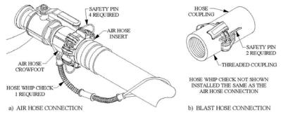
Figure 8.2 – Hose Connection Disconnect Protection
