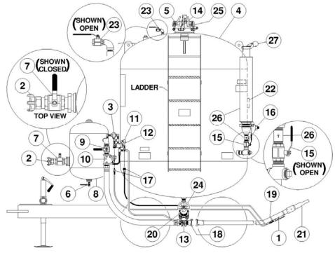
Figure 5.1 – Typical Bulk Abrasive Blaster
