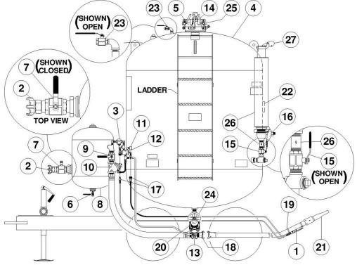
Figure 6.2 – Typical Bulk Abrasive Blaster
