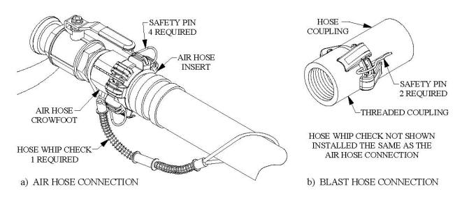
Figure 5.5 – Hose Connection Disconnect Protection
