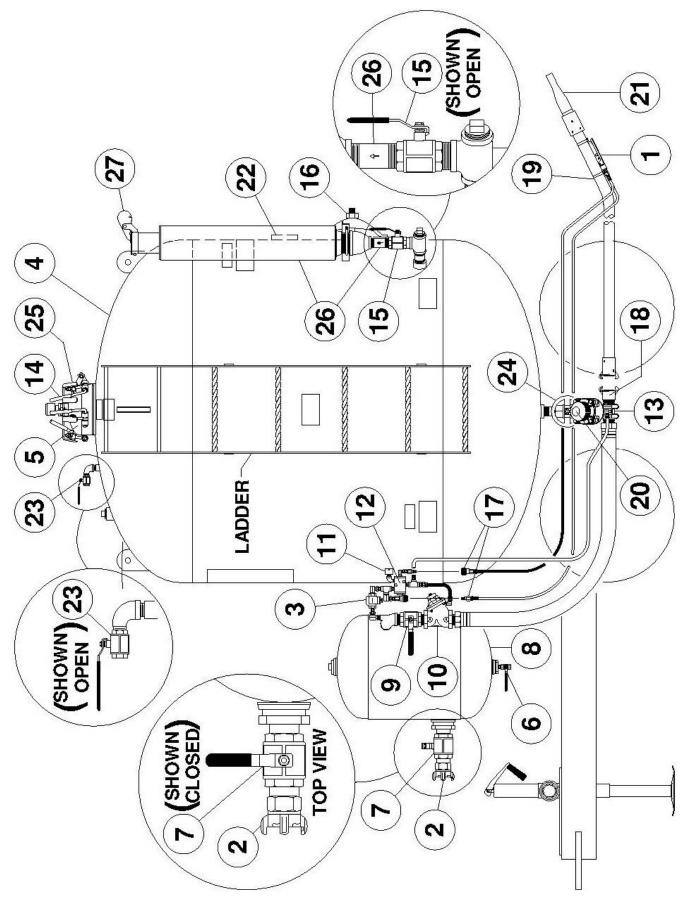
Figure 8.7 – Typical Bulk Abrasive Blaster
