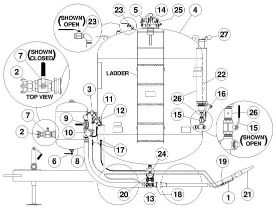
Figure 11.1 – Typical Bulk Abrasive Blaster
