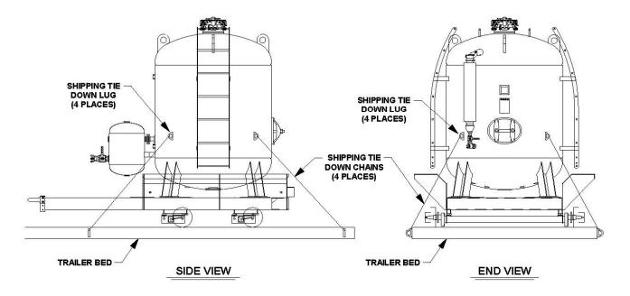
MODEL 120 & 160 TRAILER MOUNT ATTACH CHAINS TO DESIGNATED SHIPPING TIE DOWN LUGS ONLY (4 PLACES). POSITION CHAINS NOT TO CONTACT TRAILER FENDERS (4 PLACES). REMOVE WHEEL ASSEMBLIES TO INSURE THAT HEIGHT LIMIT IS NOT EXCEEDED.
