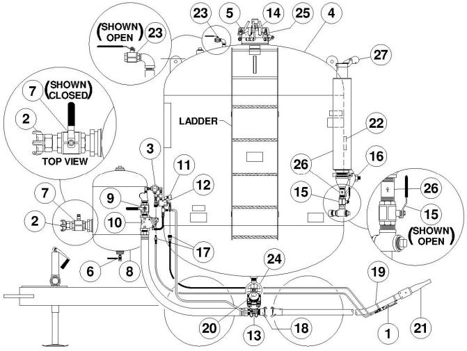
Figure 5.1 – Typical Bulk Abrasive Blaster
