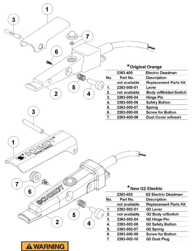
\*Electric shock hazard. To minimize shock hazard use electric deadman in low voltage applications only (12-24 volts).
