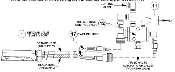
Figure 5.3 – Pneumatic Blast Control System
