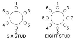
Figure 8.5 – Trailer Wheel Torque Sequence
