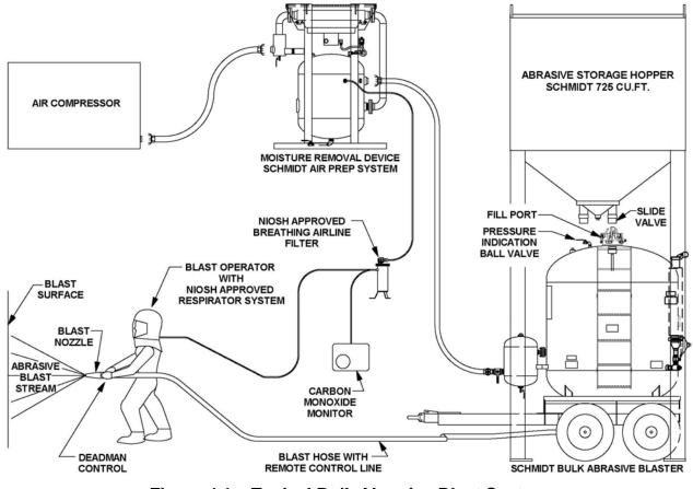
Figure 4.1 – Typical Bulk Abrasive Blast System
