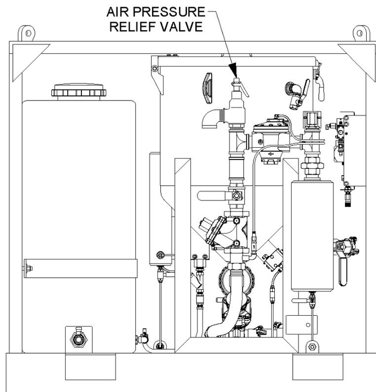
**Figure 3.11 – Suggested Location For Air Pressure Relief Valve**
