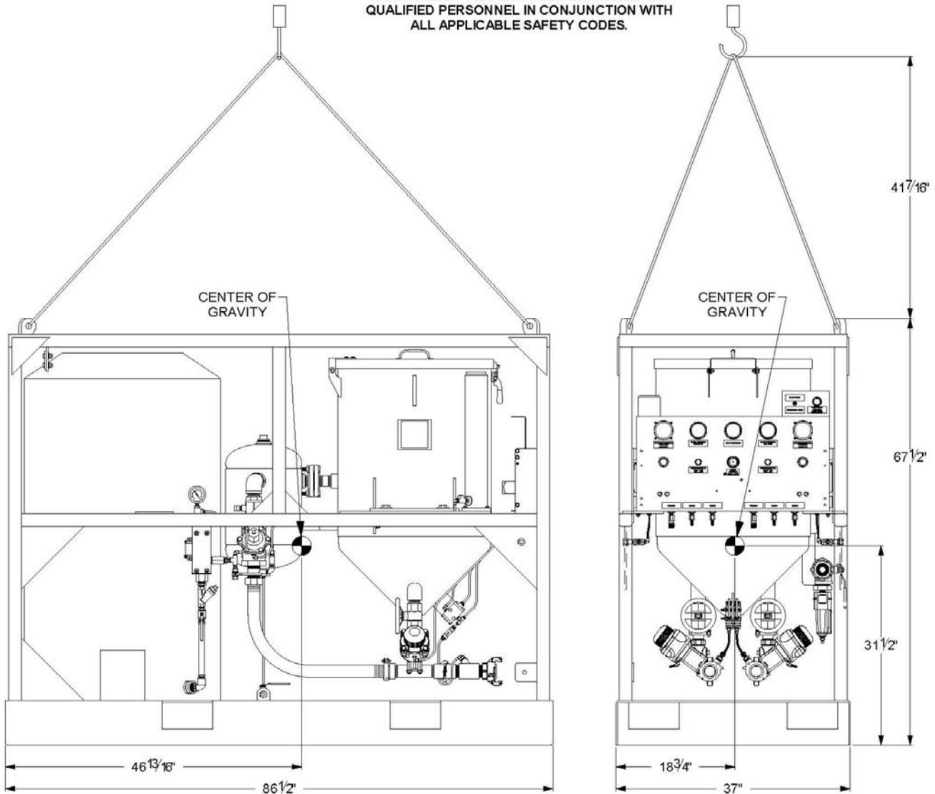
Figure 2.6(b) – Amphiblast™ 6.5 (2-Outlet) Lifting Diagram and Dimensional Data
