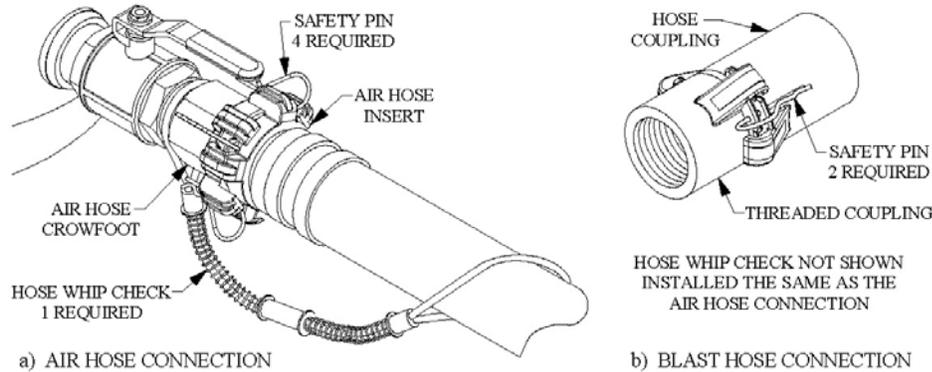
**Figure 5.4 – Hose Connection Disconnect Protection**
