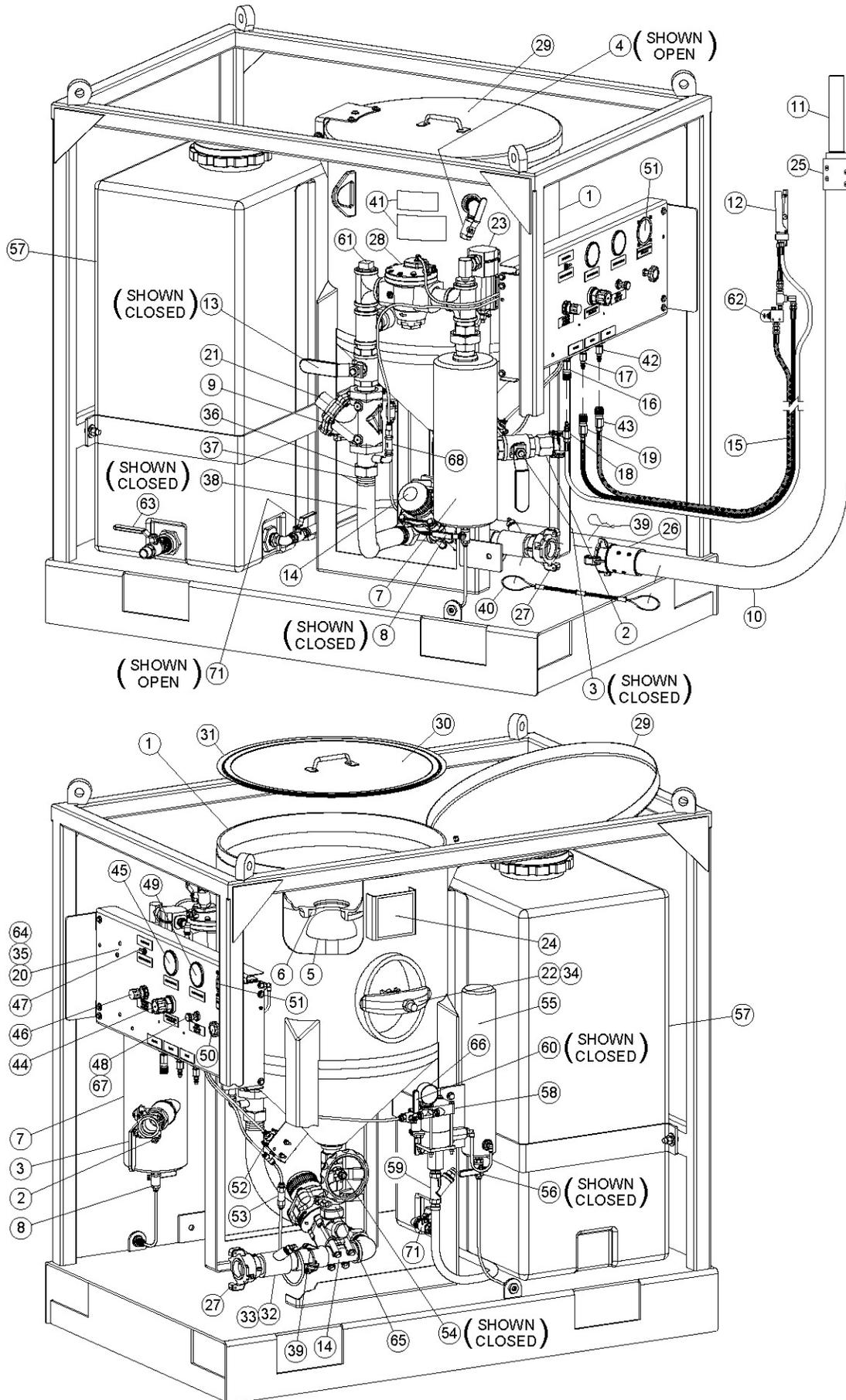
**Figure 5.1 – AmphiBlast™ With Pneumatic Blast Controls**
