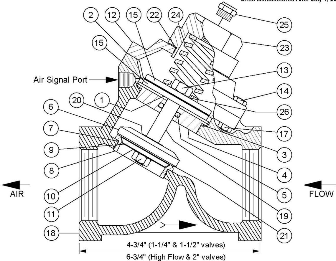
NOTE: With spring closed valve air flow is in opposite direction from arrow on valve body.
