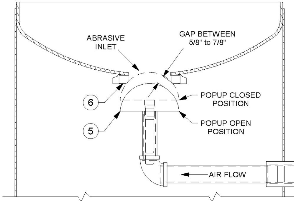
Figure 5.2 – Standard Popup Assembly & Internal Piping
