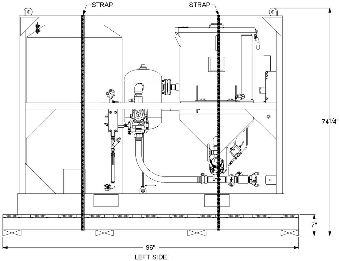
STRAP AMPHIBLAST TO PALLET AS SHOWN
