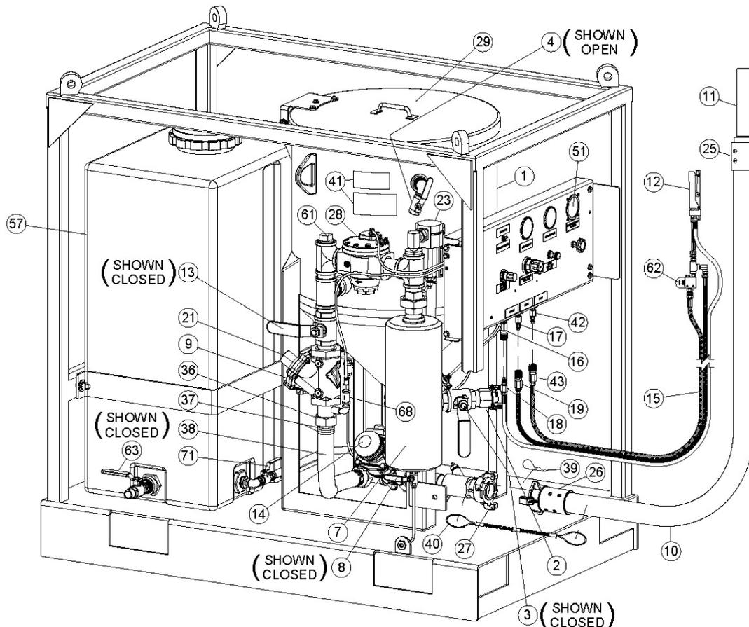
Figure 6.2 – AmphiBlast™ With Pneumatic Blast Controls
