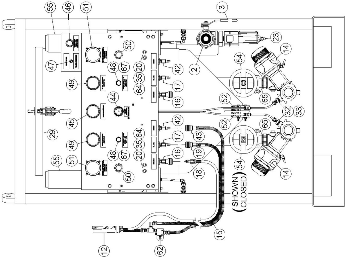
9.1(f) **AmphiBlast™ 6.5 Pneumatic 2-Outlet Control System (Right Side)**
