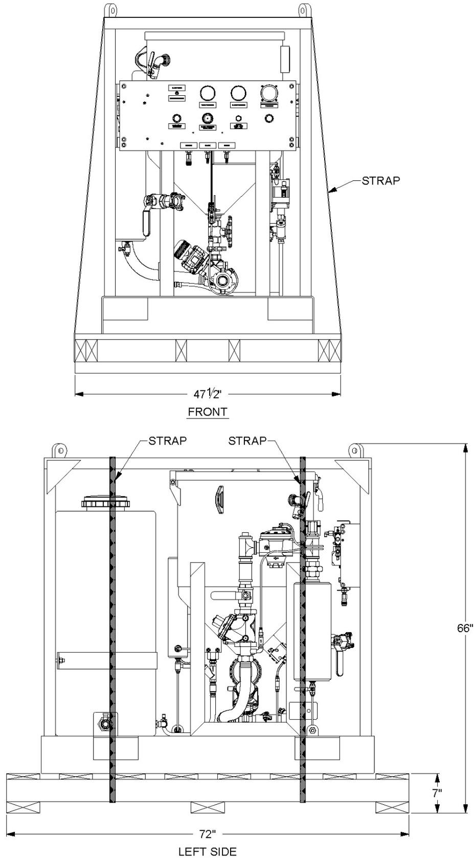
STRAP AMPHIBLAST TO PALLET AS SHOWN
