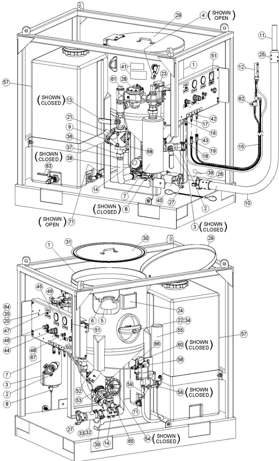
Figure 7.1 – AmphiBlast™ With Pneumatic Blast Controls
