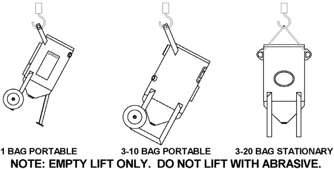
Figure 2.6(a) – Abrasive Blaster Lifting Diagram
